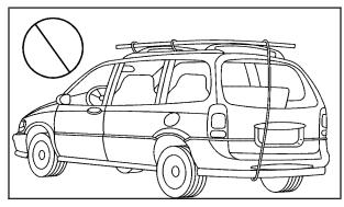
If your vehicle has a luggage carrier, you can load things on top of your vehicle. The luggage carrier has side rails attached to the roof. You can get sliding crossrails through your dealer to use for tying things down. These let you load some things on top of your vehicle, as long as they are not wider or longer than the luggage carrier.
